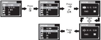
Use the  $\Im O$  or O<sup> $\oplus$ </sup> buttons to select a field, such as year, month, day, hour, minute. Use the  $\overset{\flat}{O}$  or  $\overset{O}{G}$  buttons to adjust the value in the field. Press the OK button after all fields are set.
